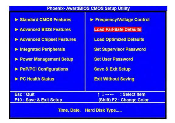
Pressing Y loads the BIOS default values for the most stable, minimal system performance.
