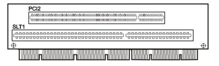
$\bigcirc$  The Riser Card has a total of 2 expansion slots, but user are only allowed to use one expansion slot, you may choose to the PCI or the ISA slot.
