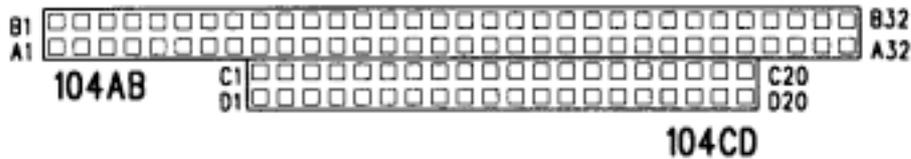
The PC/104 can support multi-pieces of PC/104 modules. This card has two connectors : one (104AB) consists of 64-pin dual-in-line header, the other one (104CD) consists of 40-pin dual-in-line header
