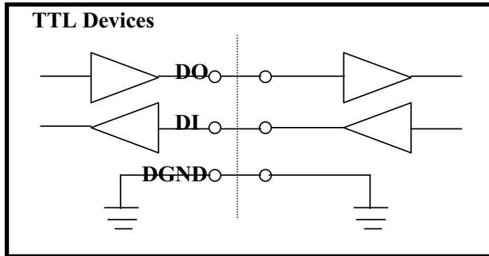
**Connection with COMS Device** – Use a pull-up resistor if you wish to interface to COMS devices. This will raise the logic high output level from its minimum TTL level of 2.4 to +5V suitable for COMS interface.
