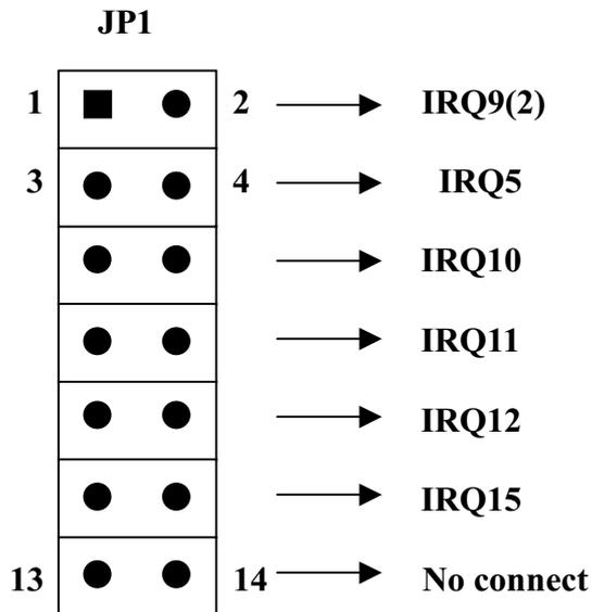
In factory jumper JP1 pin13-pin14 is installed on .
